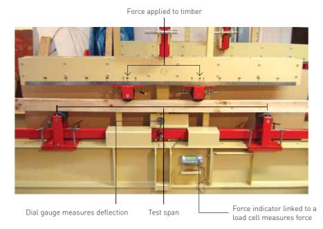
VSG (Visual Stress Grades) are sorted on the basis of visual characteristics. Visual characteristics are good for determining strength but not so good for predicting stiffness. Whereas the quality assurance checking for machine stress grades is probably more important for ensuring the strength characteristics are achieved, in the case of visual stress grades, the verification process is more pertinent for checking the stiffness characteristics.
